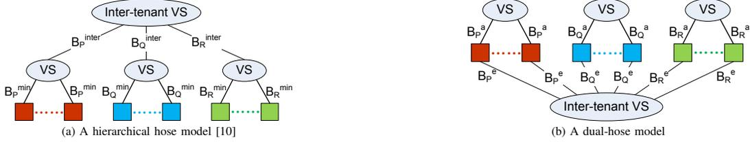
Fig. 1. Characterizing the minimum bandwidth guarantees for tenants. VMs of different tenants are marked with different colors.
