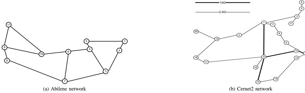
Fig. 8. Backbone network topologies
