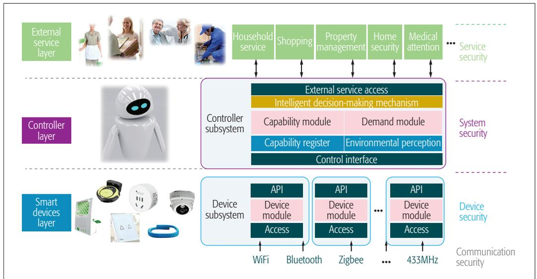
Figure 3. SDSH platform architecture.
